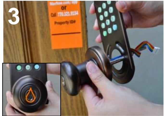
Hold the front door knob so that the keyhole has a larger opening at the bottom. Slide the 12-button faceplate onto this knob. **Tip: If right side up, keyhole opening resembles teardrop.**
