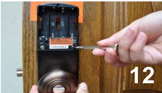
Insert the 2 shorter gold screws into the holes below the battery compartment. Tighten screws so assembly is snug to the door. **Tip: Do not to over-tighten as this may cause the unit to not work.**
