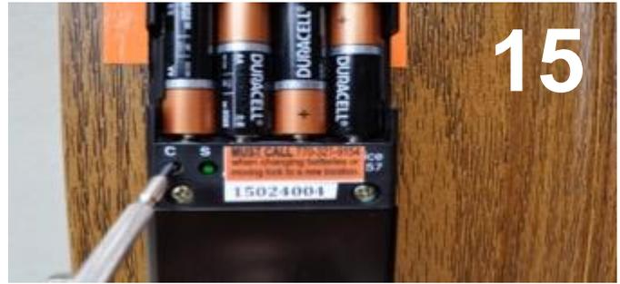
You will be instructed to press the button in the left hole. Once the green light is flashing, the Call Center will walk you through the programming sequence.
