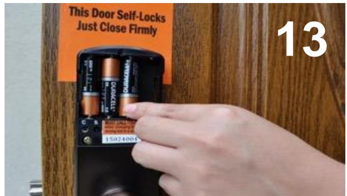
Firmly, insert 4 new "AA" coppertop batteries. The unit will automatically give an "upward" trill. **Tip: If there is no "trill" sound, remove and reinstall batteries.**
